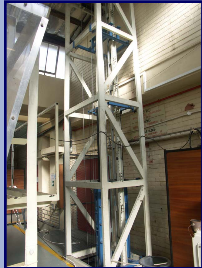
10 th Scale mine headgear for overwind/underwind simulations
