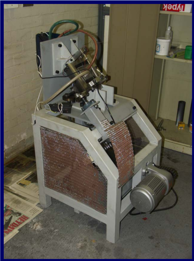
Single station mechanical hip simulator according to Paul profile
