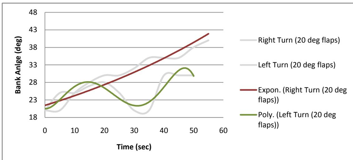
**Figure 8. Some Student Data from a Spiral Stability Flight Test**
