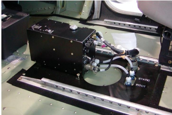
**Figure 3. MFDRS Installation on Cessna 172**
