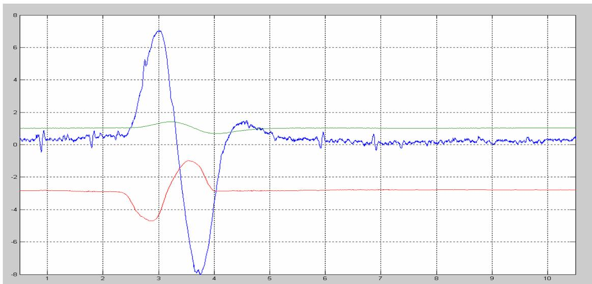
**Figure 6. Sample Flight Data: Pitch Doublet**
