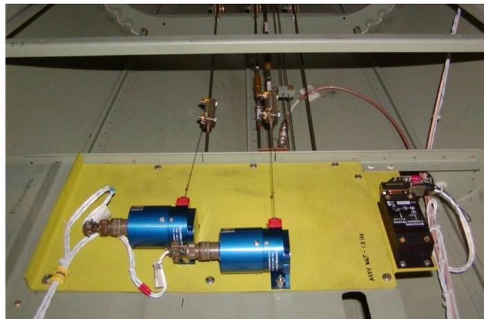
**Figure 4. Elevator, Rudder, and Magnetometer Transducer Installation**
