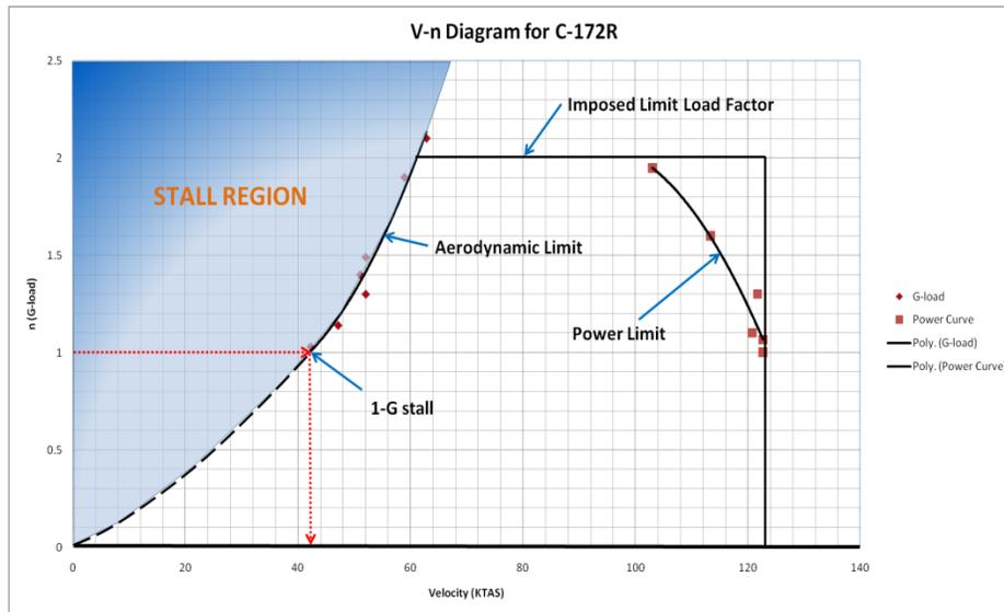
**Figure 7. Some Student Data from a Turn Performance Test**
