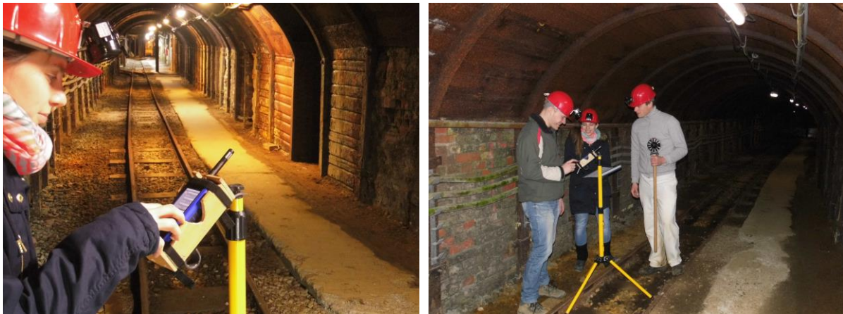
Figure 3: Ventilation survey, individually (left side) and in a group (right side)
